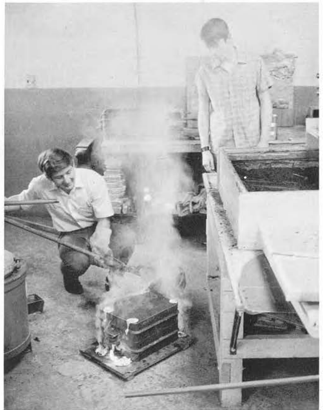
Members of a general shop class, Pat Cypher and Paul Fay, pour aluminum into a sand mold to make a casting for a pie mold.
