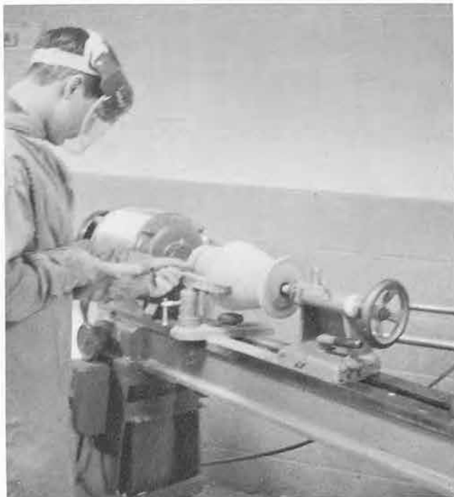
Arnold Riley is working on the wood-turning lathe to turn out a table lamp made of mahogany wood.
