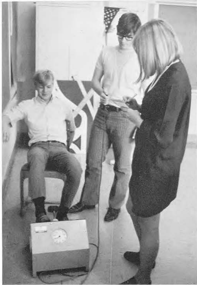
Jim Joyce tests his reaction time, the time it takes to move his foot from gas pedal to brake, on the psycho-physical testing machine. Aiding in the test are Jo Utter and Byron Gray.
