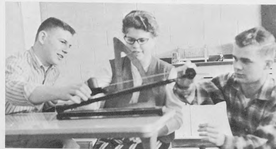
J. Stanke, S. Soma, and E. Sickenberger prove that length divided by height equals mechanical advantage.
