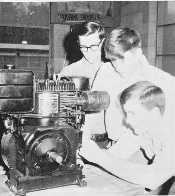
BY ADJUSTING THE CARBURETOR OF THIS SMALL ENGINE in basic shop, Scott Smith, Larry McFaul and Arnie Platt gain understanding of the operation of more complicated engines.
