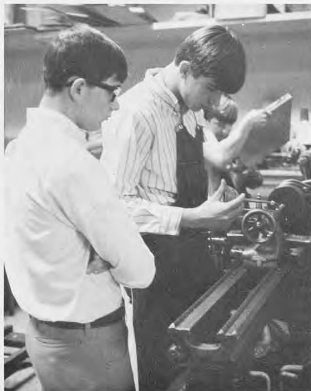
USING THE METAL LATHE , Tom Knox and Bob Fish are turning a half-inch rod into a center punch during a general shop class.
