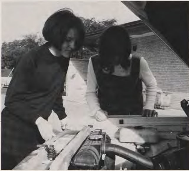
JANE WALKER AND SANDY STIEVE are removing the air filter to adjust the carburetor before they start a period of practice driving.
