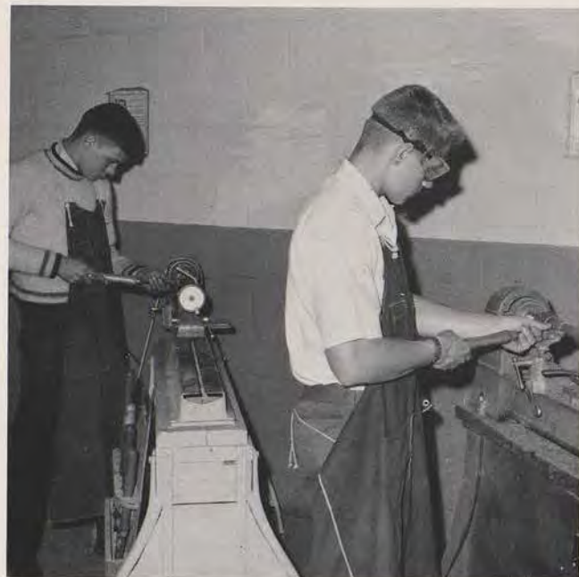
ED FITZGERALD AND MIKE MARSLANDER are working on the lathe, turning a leg for the bookrack they are making in advanced woods class.
