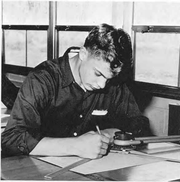
Charles Meltz is using a drafting machine to make a mechanical drawing.
