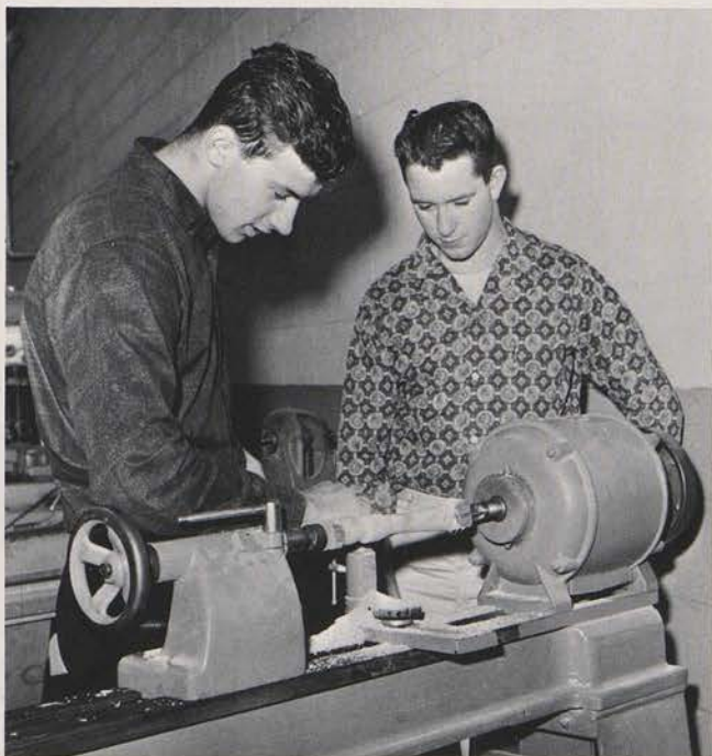
In the industrial arts course boys learn the art of making fine furniture, and here Dale Stukel and Tim Tobin are turning a table leg on the wood lathe.
